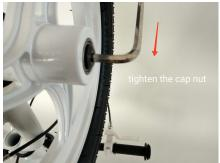
Slide the first wheel on, then the second, insert cap nuts and tighten both sides.
