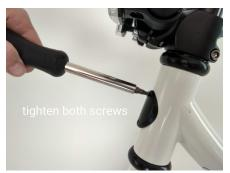
Slide the stem and handlebars onto the fork, lightly tighten, attach headset spacer and cap nut, tighten headset cap bolt making sure there is no play or restriction, line up handlebars with the frame.
