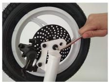
Drop the front wheel into place in the forks. Slide the front axle through the fork, attach the other nut and tighten both sides.
