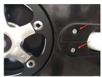
The guard has 3 components, back, upper and lower, the back is pre-installed. Attach the bottom guard and locate the central screw, ensure that it's clipped th the back, tighten screw, repeat for the upper guard.
