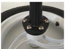
Insert the six adapter bolts, make sure to protrude one bolt for installation guidance, attach to the wheel counter adapter, tighten each bolt in opposite sequence, a cordless driver will speed this process.
