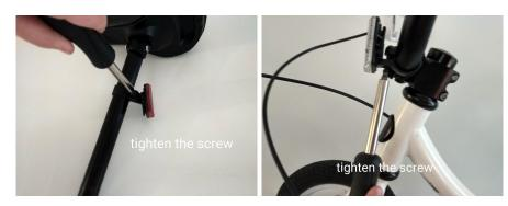
Insert the screw and tighten.
