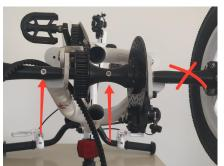
Line up the hole on the adapter/axle, insert the bolt and tighten with 4mm hex, do not insert a bolt on the right side adapter.
