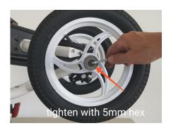
Insert the small cap nut & washer and tighten with 5mm hex, repeat for the other wheel.
