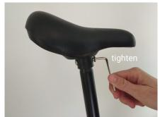
Line up the holes in the post and saddle, insert bolt, attach nut and tighten, please observe the minimum insert mark for the saddle height.
