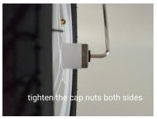
Slide on the first wheel, either side, slide on the second wheel, place the washer on the nut and screw onto the axle, tighten cap nut.. Make sure both wheels spin freely.
