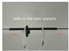
Insert the bearings into the large frame holes, place the central spacer in position over the holes, slide on the two outer spacers, use them to tap the bearings into place.
