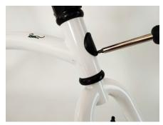
The badge is secured with two small screws, undo both, remove the badge to expose the limiter.
