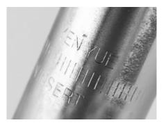
Minimum insertion mark on the seat posts.
