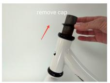
Undo both screws on the badge, remove headset cap, loosen both stem bolts, remove stem with handlebars attached, remove top headset components, (plastic washer and aluminium cap).
