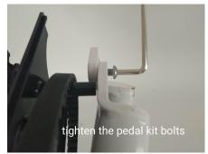
With the outer belt guard covers removed, insert the pedal kit onto the frame making sure the belt is inside, hook the belt over the guard plastic pin. Line up the pedal kit bolt holes with the frame holes, insert 6mm bolt and tighten, repeat on the opposite side.
