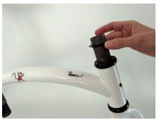
Undo steering limiter bolt, slide forks out, flip frame and reinsert forks, slide the headset cap and plastic washer back on.
