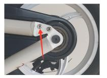
Screw the upper section together, then the lower section, finally insert the bolt into the pin and tighten.
