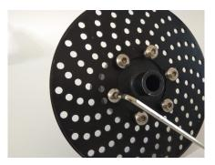
Insert the frame bearings both sides, the inside edge of the bearing flush with the frame. Attach a rotor to the central unit, tighten bolts in opposite sequence.
