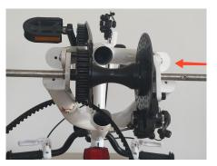
Screw the freewheel onto the central unit, slide the central unit into place using the rotor/caliper as the guide, hook the belt to the position in the arrow, slide in the long axle.
