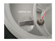
There are reflectors for both wheels in bicycle mode; Place a washer then slide a bolt through the reflector hole, insert in the wheel gap as shown, on the reverse side add the washer and nut, tighten, you may need the addition of a spanner for the nut.
