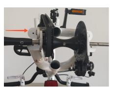
Line up the holes on the central unit, insert the bolt and tighten with 4mm hex, fit the belt by hooking over the freewheel and feeding over the front pulley. Slide on the left hand wheel & adapter.
