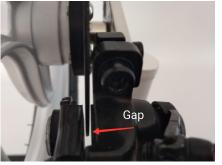
The front and rear calipers have two adjustment bolts to centre the disk. Very small adjustments are needed; loosen both bolts and manually centre whilst checking the disc moves freely in the gap between the pads by rotating the wheel.
